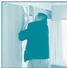
The combination of a sheet and solid core door will support the entire body weight off the ground.
